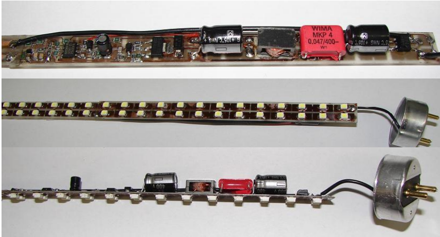
Bottom view PFC LED tube board (partial view, total amount of LEDs: 104- 120)
